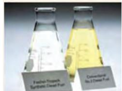
*Side-by-side comparison of FT synthetic fuel and conventional fuel. The synthetic fuel is visibly cleaner, being as clear as water because of a near-absence of sulphur and aromatics.*
